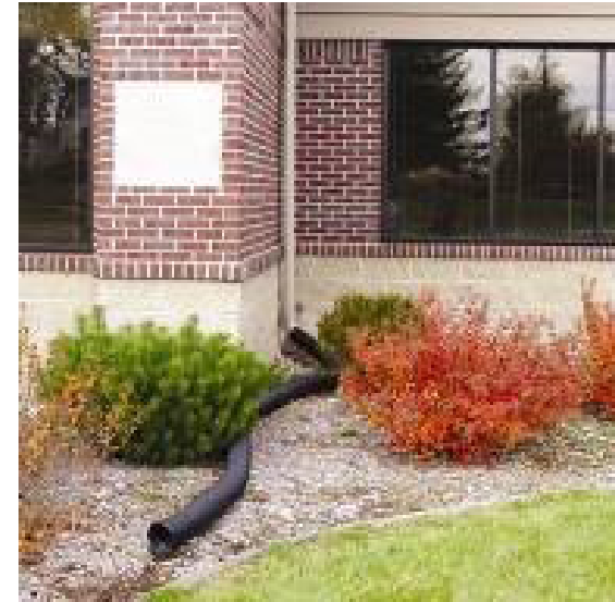
Figure 4.4.2 Downspout Disconnects to Pervious Areas (Source: Center for Watershed Protection)
