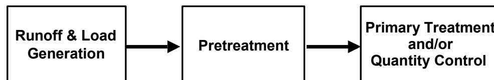
Figure 4.1.6-1 Generalized Stormwater Treatment Train
